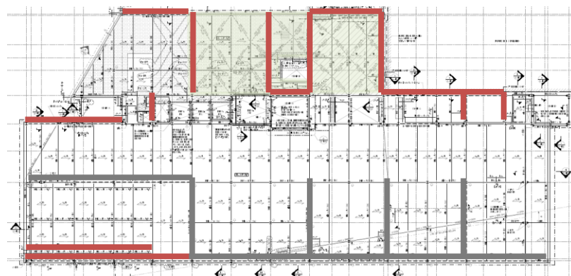
Figure 9: Level 5 Framing Plan Showing Lateral System (S-105) — Lateral Braced Frame — Gravity Truss that Contributes to Lateral System — Floor System with Diagonal Bracing
