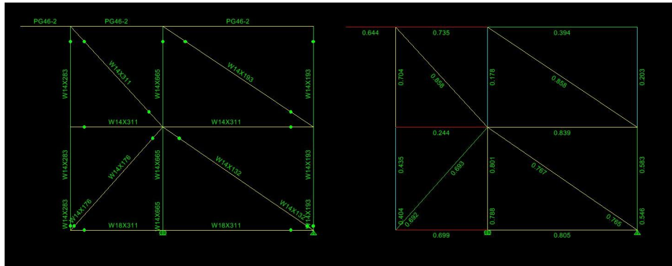
Figure 35: Truss H Modeling Input and Design Results
